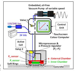
The air at atmospheric pressure, present in the pores of the concrete underneath, flows through the cover concrete into the inner chamber, raising its pressure  $P_i$ . The rate of increase of pressure  $P_i$  is directly linked to the coefficient of air-permeability of the cover concrete.
